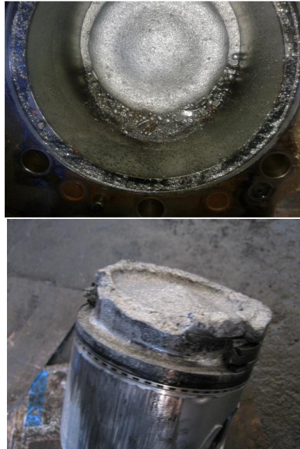
Shape 2- severe failure of piston (made in Iran) before deadline
